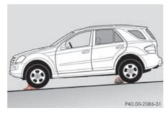
Securing a vehicle on slight downhill slopes (example illustration)
