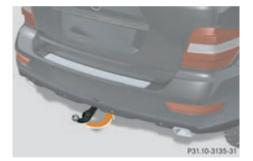
Press the ball coupling in the direction of the arrow by hand until it engages behind the bumper.
