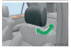
▶ Push or pull the head restraint in direction of the arrow.
