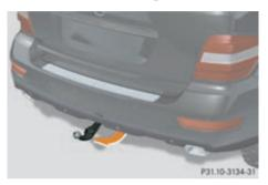
▶ Press the ball coupling in the direction of the arrow by hand until it engages in a vertical position.
