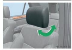
▶ Push or pull the lower edge of the head restraint in direction of arrow.
