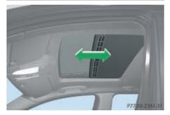
The cover functions as a sunblind. When you open the sliding/tilting sunroof, the cover moves back with it.
