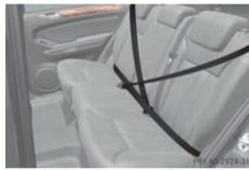
If the rear seats are not occupied, insert the belt tongue on the outer seat belts into the buckle of the opposite seat belt. This increases the restraining effect of the rear seat backrests.
