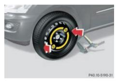
► Slide the emergency spare wheel\* or the spare wheel onto the centring pin and push it on.
